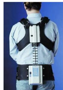
Figure 3.1. A worker wearing a lumbar motion monitor (LMM).
