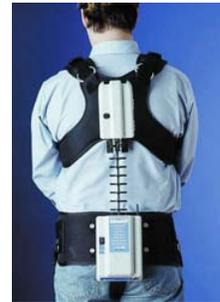
Figure 3.1. A worker wearing a lumbar motion monitor (LMM).
