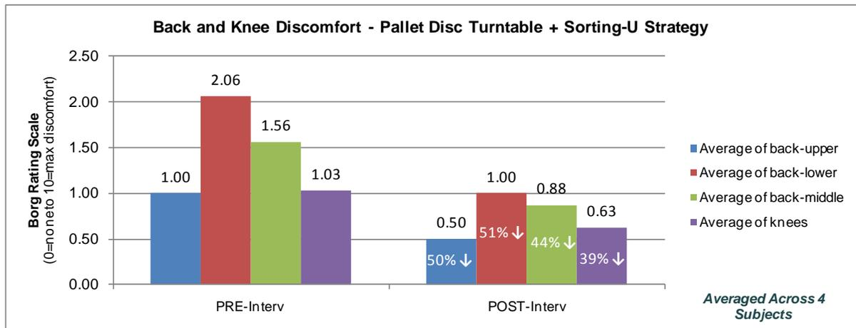
**Figure 4.2. PRE- vs. POST-Intervention Discomfort Results<sup>1</sup>.** Using the pallet disc turntable + sorting-U pallet layout strategy in the back room for pallet breakdown.
