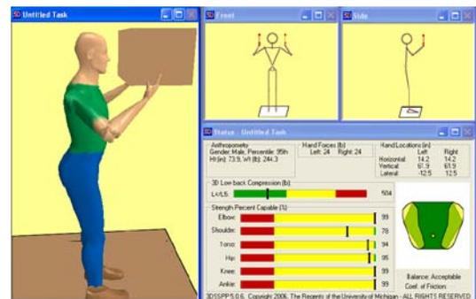
Figure 3.2. Screen capture of the 3DSSPP application. In the illustration above, a two-handed lift of 48 lbs is modeled using the anthropometry of a 95% male.
