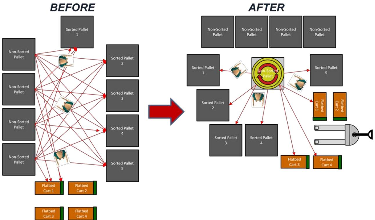
**Figure 4.1.** Pre- vs. Post-Intervention Illustration of Back Room Pallet Breakdown and Sorting Strategy. The layout on the left depicts the pre-intervention strategy and the layout on the right depicts the use of the pallet disc turntable and sorting-U pallet layout strategy in which stock clerks downstack from the same pallet.
